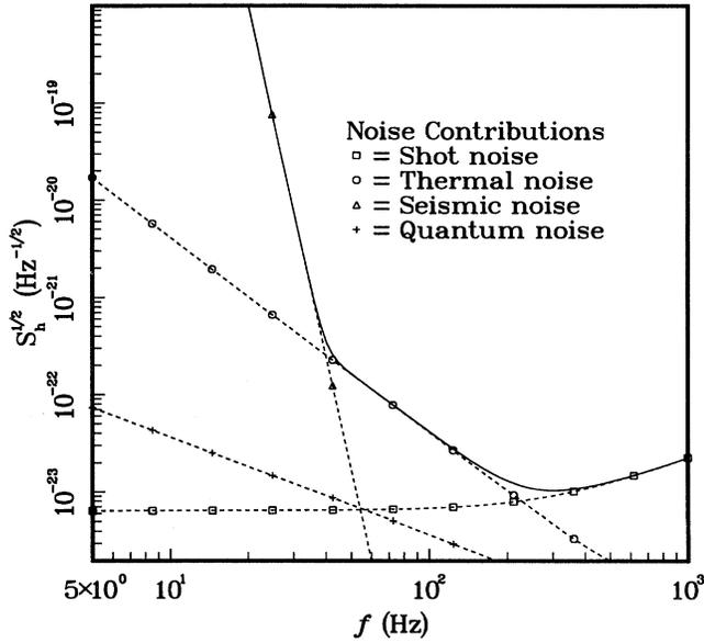
FIG. 1. The noise power spectral density (PSD)  $S_h(f)$  for the (anticipated) initial LIGO interferometers configured for standard recycling with a knee frequency of 300 Hz. The solid line shows the total PSD, while the dashed lines show the important physical limits and environmental influences that contribute to the total. For more detail, see Sec. IV A and Table II.
